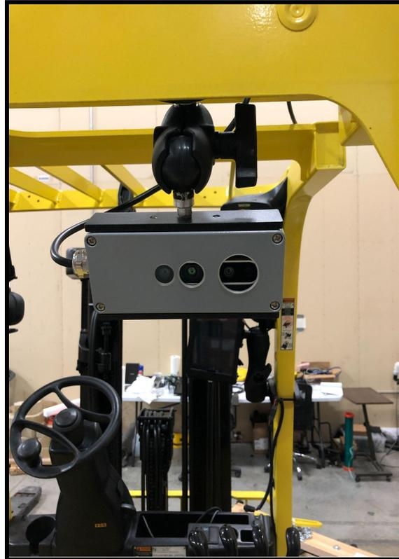
The gateway mounted the sidebar of a vehicle cage.
